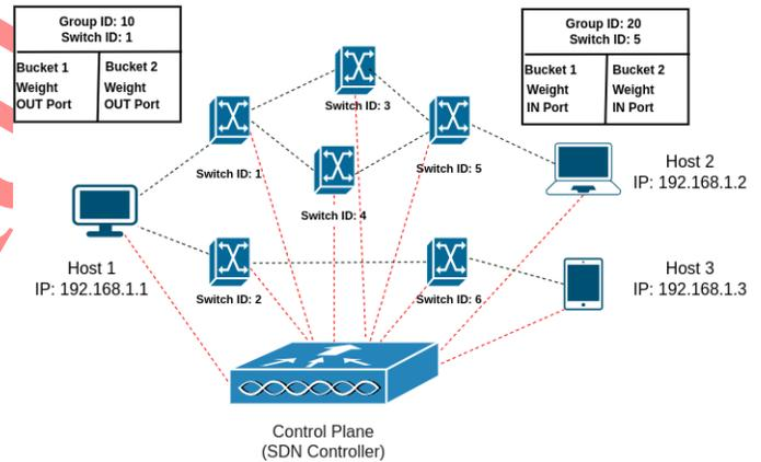
Fig. 1: Schematic Architecture of Traffic Management using Group Tables in SDN-Enabled 5G/6G Networks.
